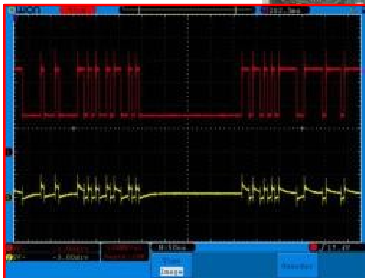
Can Network signal amplified on the oscilloscope
